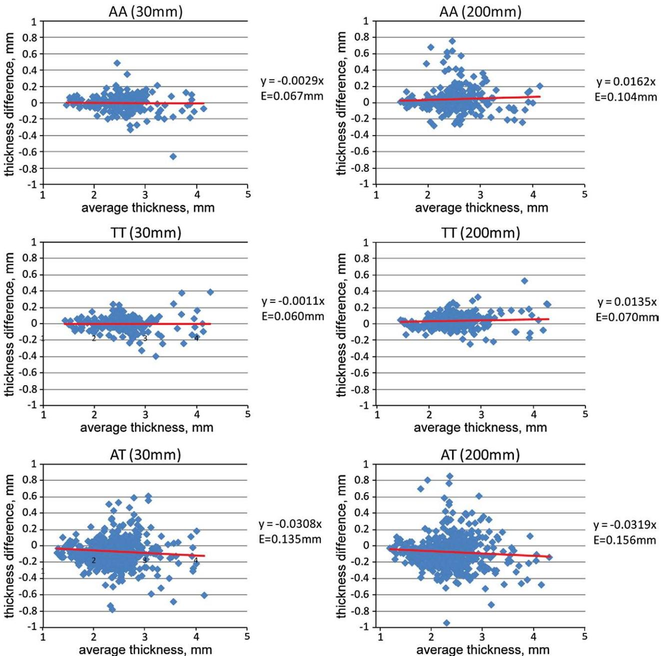
Fig. 8. Scatter plots of regional cortex thicknesses measured within Allegra scanner (AA\_\*), within Tim Trio scanner (TT\_\*) and between the two scanners (AT\_\*) with smoothing distances 30 mm and 200 mm; E represents the mean absolute thickness difference.
