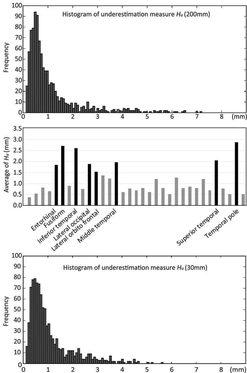
**Fig. 4.** Regional underestimation distances obtained with default N3 smoothing distance of 200 mm: histogram of all distances (top) and average distance per region (middle); highlighted bars represent values larger than 1.5 mm. Histogram of underestimation distances at 30 mm smoothing distance (bottom).
