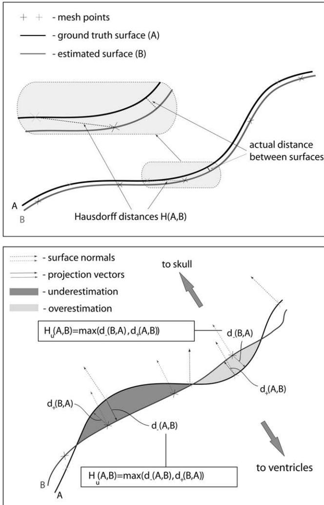
**Fig. 1.** Due to finite sampling rate, Hausdorff distance overestimates the distance between surfaces (top). Evaluation of surface underestimation  $H_u$  and overestimation  $H_o$  distances (bottom).
